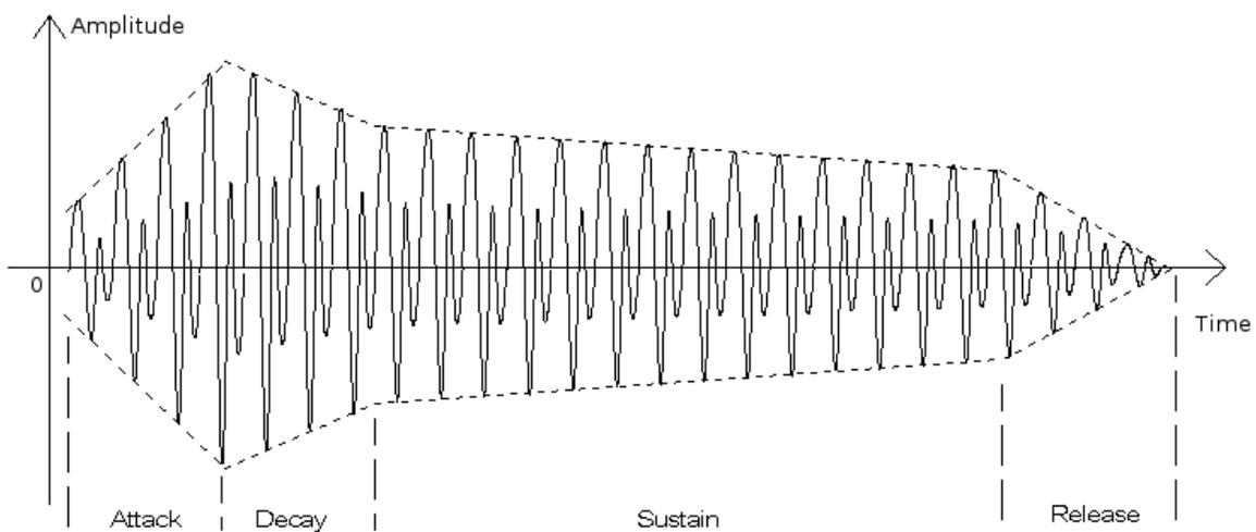
Figure 5.5: The looped sample from Figure 5.4 modulated with the ADSR envelope<sup>14</sup>.
