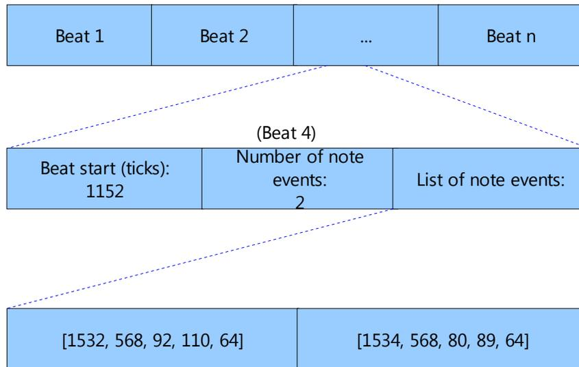
Figure 5.9: Structure of the output of Stage 1
