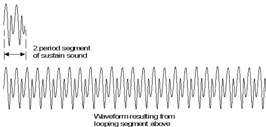
*Figure 5.4: A sampled sound segment and the same segment looped<sup>13</sup>.*
