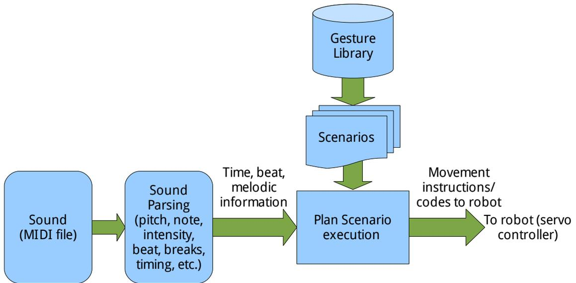
Figure 5.1: The block diagram of the proposed system
