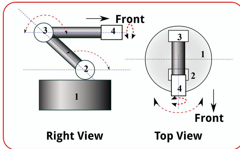
Figure 5.17: Configuration of the custom Lynxmotion robot.
