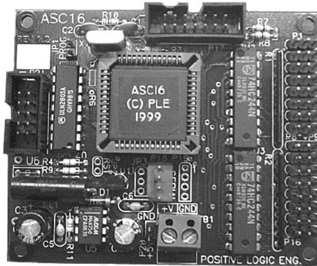
Figure 5.24: The ASC16 servo controller board<sup>19</sup>.
